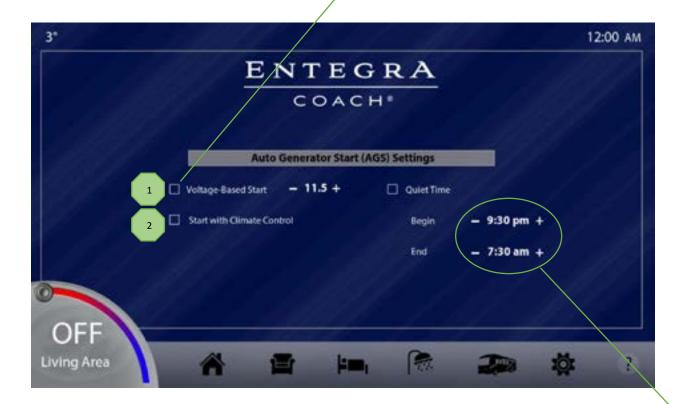
Quiet Time – Specific time settings set by the user to determine when the generator will not run to eliminate unwanted noise caused by the generator. Tap the +/- keys to control the hours that the generator will not run.
