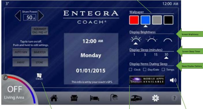
Locks the screen for 15 seconds to allow time for cleaning.
