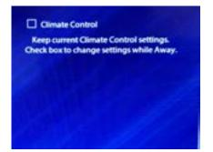
If the Climate Control box is checked, but neither A/C nor Heat box is checked, then all Climate Control equipment will turn off.
