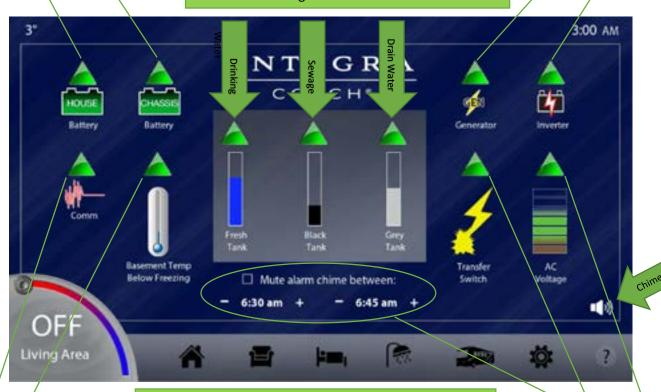
Tap the box to enable Alarm Chime Mute and press the +/- keys to select the hours you would like it silenced.
