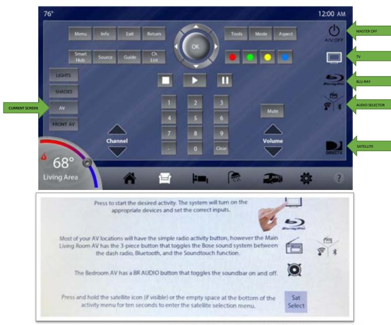
Press to select the installed satellite receiver - selected device is highlighted in red. The system will add the satellite to your activity selections. Press "SAVE" to finish.
