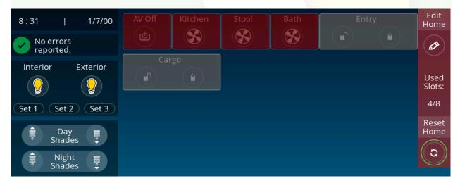
Fan Controls – Press and Hold any Fan button to bring up the Fan Dialogue screen.
